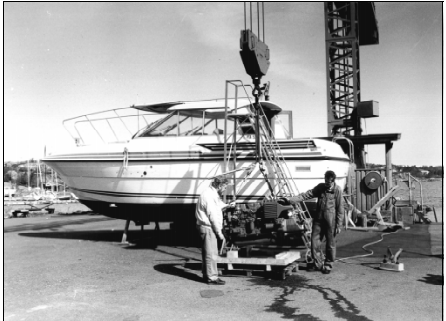
Preparing for a differential torsional vibration measurement at the Volvo Penta Marine Test Center, in Gothenburg, Sweden
